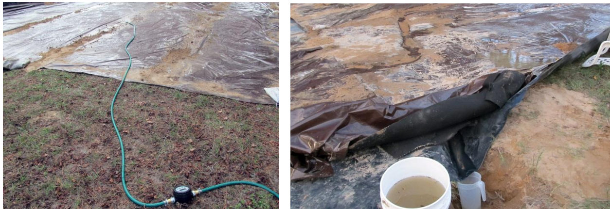
Figure 2. In-line flow meter measuring total simulated rainfall viewed from top side of test pad. Figure 3. Lower corner of test pad at end of collection trench where cover-penetrating quantity is collected in a graduated pitcher. Most fluid is shed as runoff by this continuous barrier ADCM.
