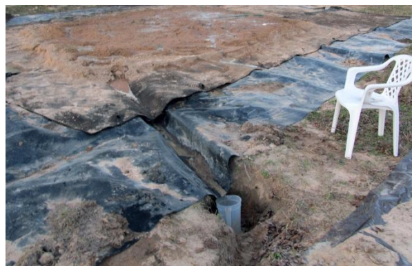
Figure 4. Green waste after breakthrough, allowing 100% rainfall to enter collection trench.
