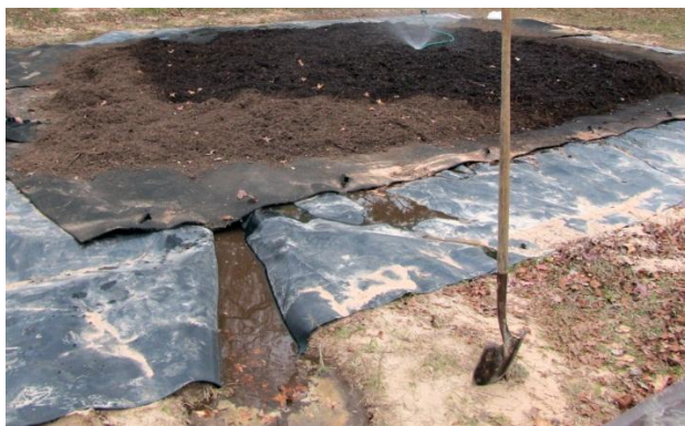
Figure 4. Green waste after breakthrough, allowing 100% rainfall to enter collection trench.
