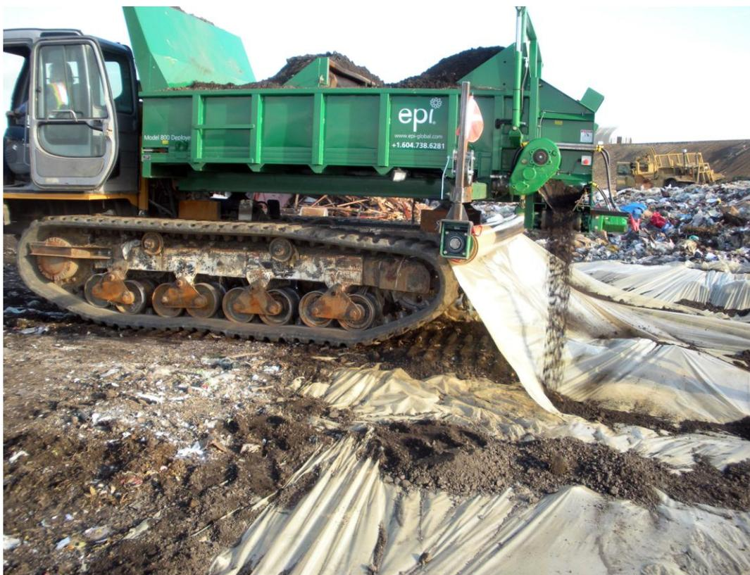
**Figure 4 – Photo of Model 800 Deployer with focus on ballast placement.**
