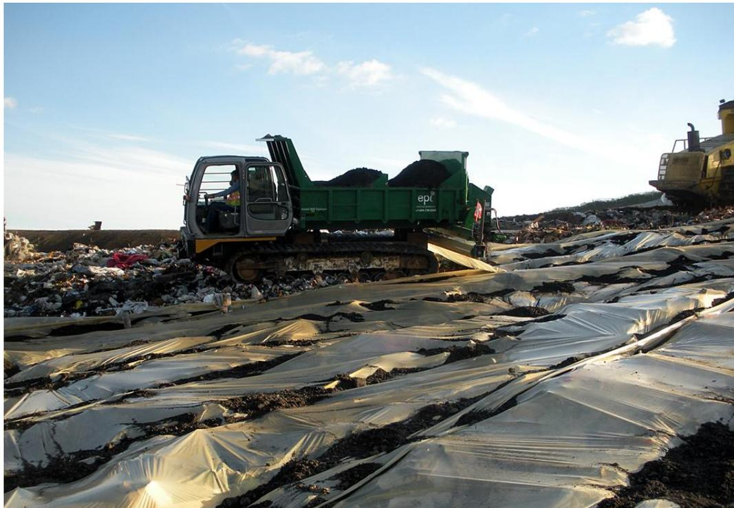
**Figure 2 - The EPI Model 800 Deployer at Puente Hills, a track mounted self-propelled film and ballast deploying device with excellent capability for efficient movement and coverage.**
